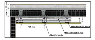
Fig. 2. Single frame plasterboard false ceiling.
