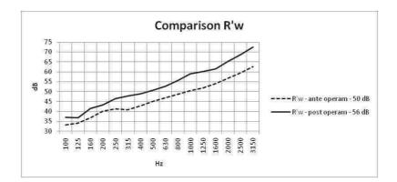
Fig. 3. Airborne sound insulation - Comparison
